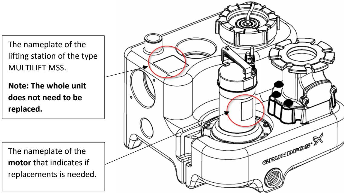
2. Check the nameplate of the **lifting station unit**:
