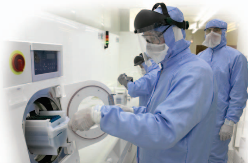
Production Technician Per Henriksen is busy drying a cassette • containing silicon discs.
