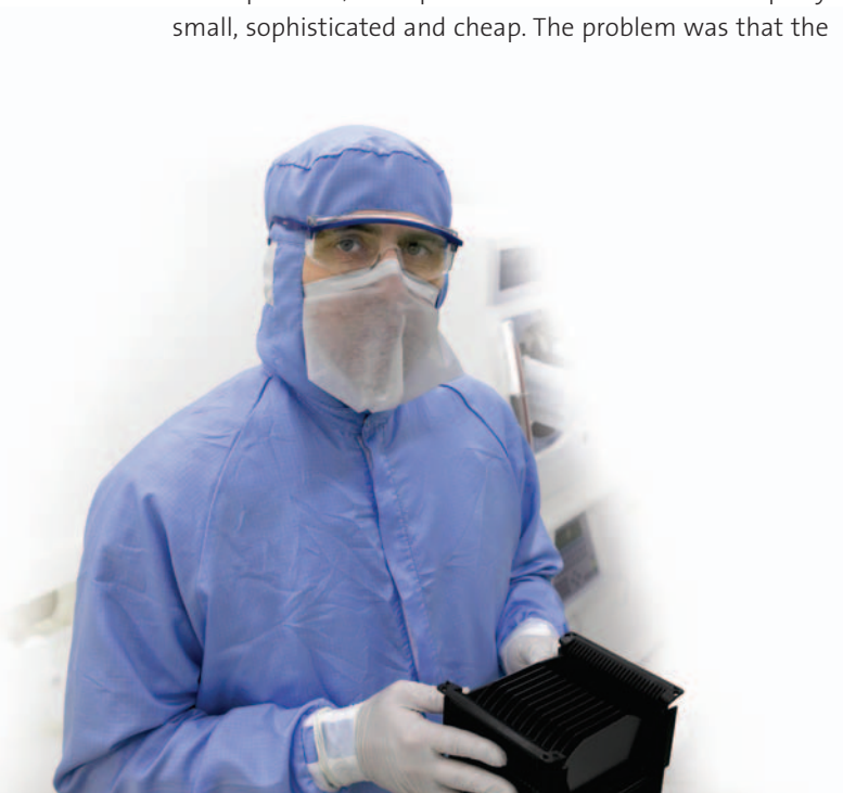
• Here, project manager Gert Friis Eriksen shows a cassette containing silicon discs. Some 800 microchips can be produced from each disc.
