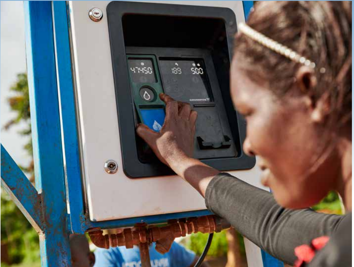
Bugoba villager Annet Kasukya uses her WaterCard (topped up with water credits) to buy 20 litres of water at a Grundfos AQtap water ATM.
