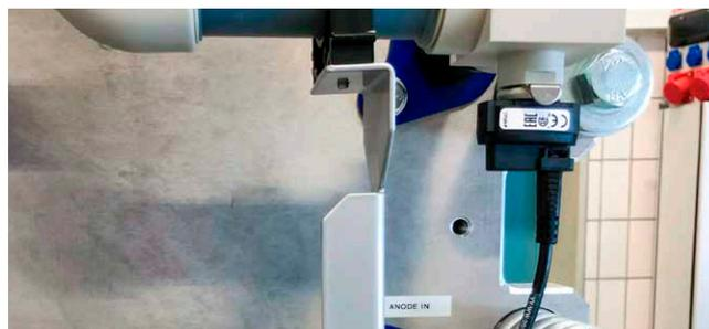
*The Relative Pressure sensors, where the stack inlet and outlet in terms of pressure and temperature are measured.*
