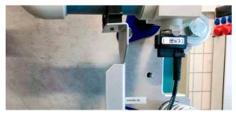
The Relative Pressure sensors, where the stack inlet and outlet in terms of pressure and temperature are measured.
