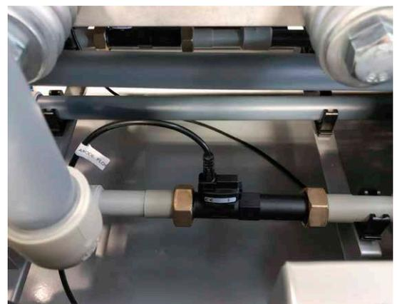
*The Multi Flow sensor, where the flow and pressure are measured. The sensor is integrated into the hydraulic system.*
