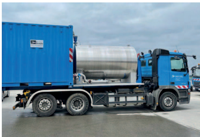
Mobile pressure boosting system with container and water tank with 10 m 3 capacity. The entire pump system is always on board and ready for action.
