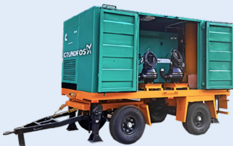
Mobile pumping station
