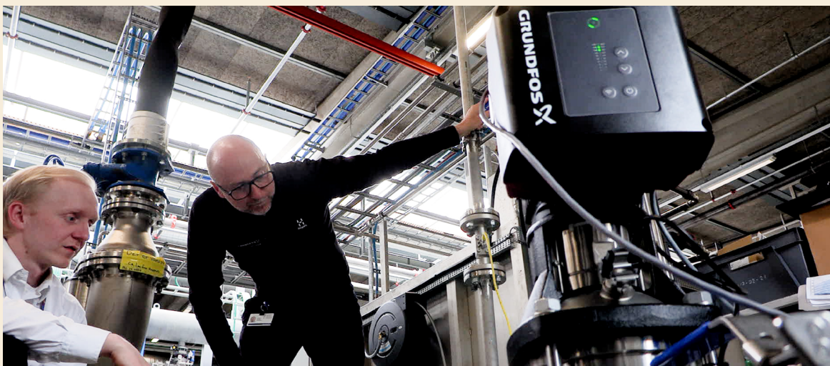
Phillip Hjelmeborn Kaae, Lead Application Manager for Grundfos (left) and Robert Guilford validate flow estimation algorithm. The enhancement compensates for differences in fluid properties between water and dielectric fluids, ensuring accurate flow estimation across cooling applications.
