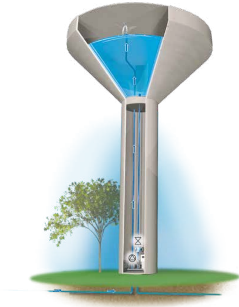
Water tower with booster set and control valve
