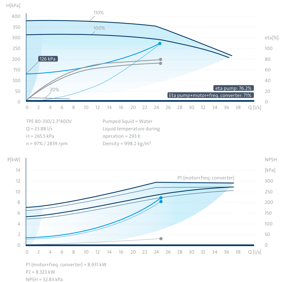
Figure 3.6.1.1 variable primary pump curve based on duty point
