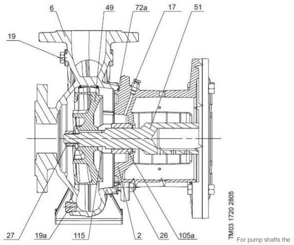
stainless steel and steel parts are friction welded together.
