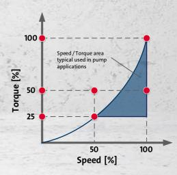
Three points of related losses and shaded area of interest for pump manufacturers when calculating the EEI (Energy Efficiency Index) of a pump unit
