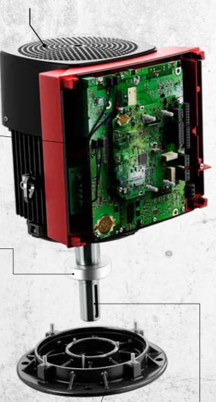
Shafts ends are available with smooth, open or closed keys.
