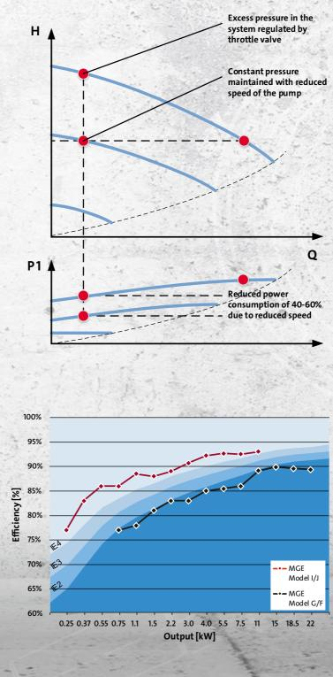
Adjusting the speed of the pump based on demand, rather than throttling the system flow with a valve, results in:
