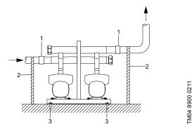
Fig. 6 Example showing the position of expansion joints, pipe supports and mounting bolts
