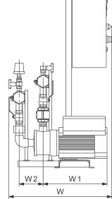
Fig. 12 Hydro Multi-B booster system with three CM, CME pumps
