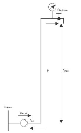
Fig. 9 Calculation of required outlet pressure
