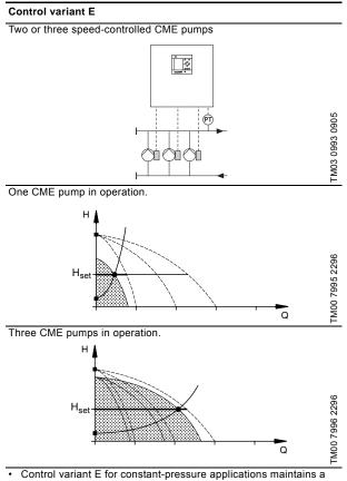
Control variant E for constant-pressure applications maintains a constant pressure through continuous adjustment of the speed of the pumps.
