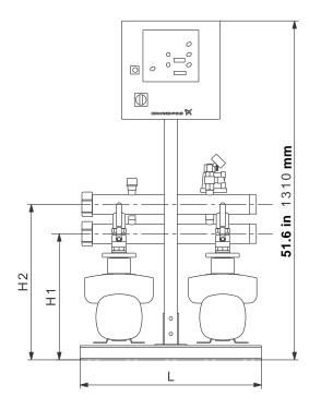
Fig. 13 Hydro Multi-B booster system with two CM, CME pumps
