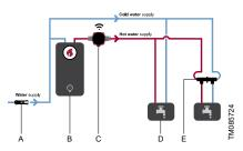
Diagram of ALPHA COMFORT SYSTEM installation
