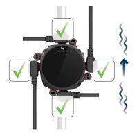
3. Insert and cross-tighten the screws.
