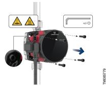
2. Turn the pump head to the desired position.
