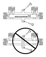
Correct installation of thermal bypass valve (mounting hardware not included)
