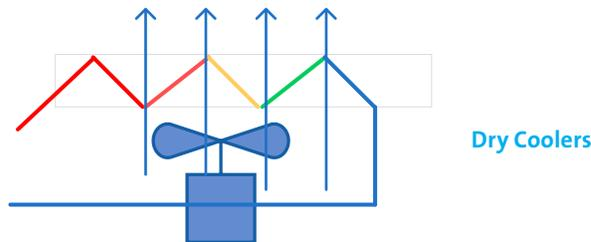
Dry coolers are used either as a free cooler or to cool the condenser in a refrigeration system.
