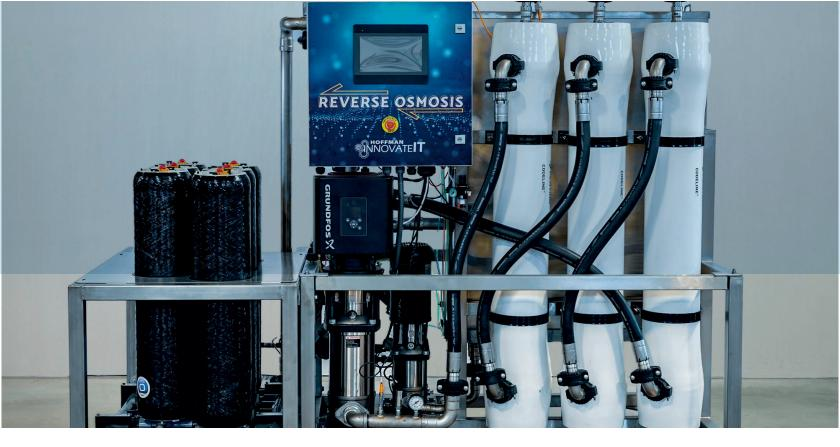
installation. innovateIT's RO system also includes built-in diagnostics and maintenance data displayed on a user-friendly touchscreen interface, providing detailed history of operating hours, cycle counts, faults and more to support both maintenance and troubleshooting minimizing downtime.
