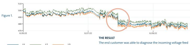
The end customer was able to diagnose the incoming voltage feed issue using an MP 204 and Grundfos Utility Connect (GUC) restoring plant operations.
