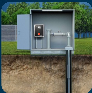
Groundwater Intake/ Borehole pumping
