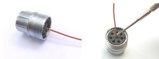
Fig. 27 Inserting the crimped cable in the connector
