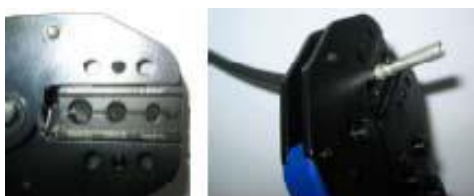
Fig. 20 DC cable crimping
