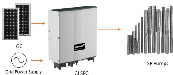
Fig. 1 GI SPC system with solar package module
